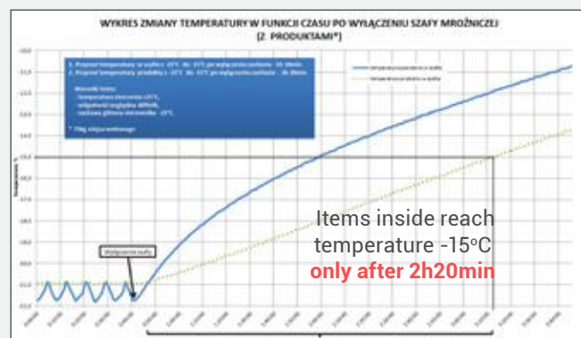
Autonomy for upright freezer of PREMIUM line (ambient temp. 25°C)
